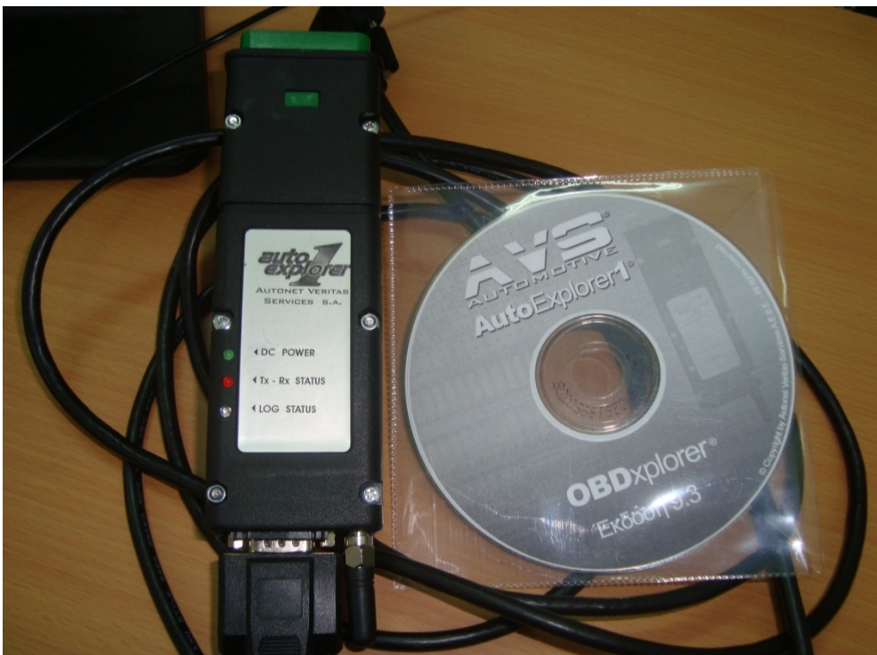
Figure 4 :Motor self – Diagnosis unit Autoexplorer 1 with 16-pin data link connector
