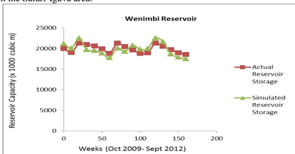
Figure 5: Simulated and Actual Capacity of Wenimbi Reservoir, October 2009 to September 2012.
