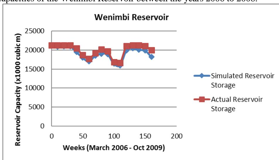
Figure 4: Simulated and Actual Capacity of Wenimbi Reservoir, March 2006 to September 2009.
