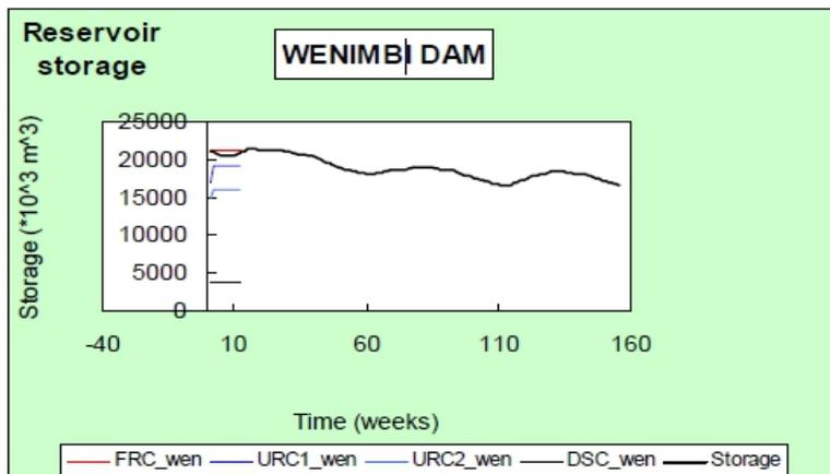
Figure 9. Wenimbi Reservoir storage at peak demand (Marondera Town water supply connected and 75% irrigation efficiency)
