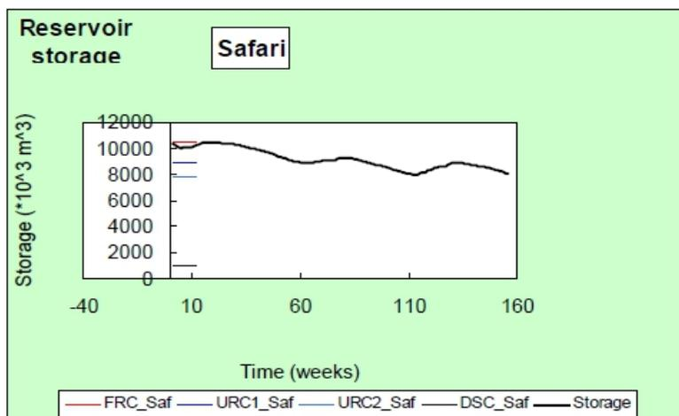
Figure 10. Safari Reservoir storage at peak demand (Marondera Town water supply connected and 75% irrigation efficiency)
