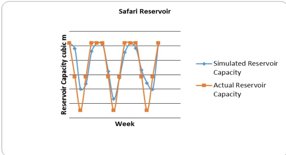
Figure 7: Safari reservoir simulated and actual capacity curves, irrigation efficiency at 75% from October 2006 to September 2009.
