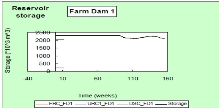
Figure 11. Eirene Farm Reservoir 1 storage at peak demand (Marondera Town water supply connected and 75% irrigation efficiency)
