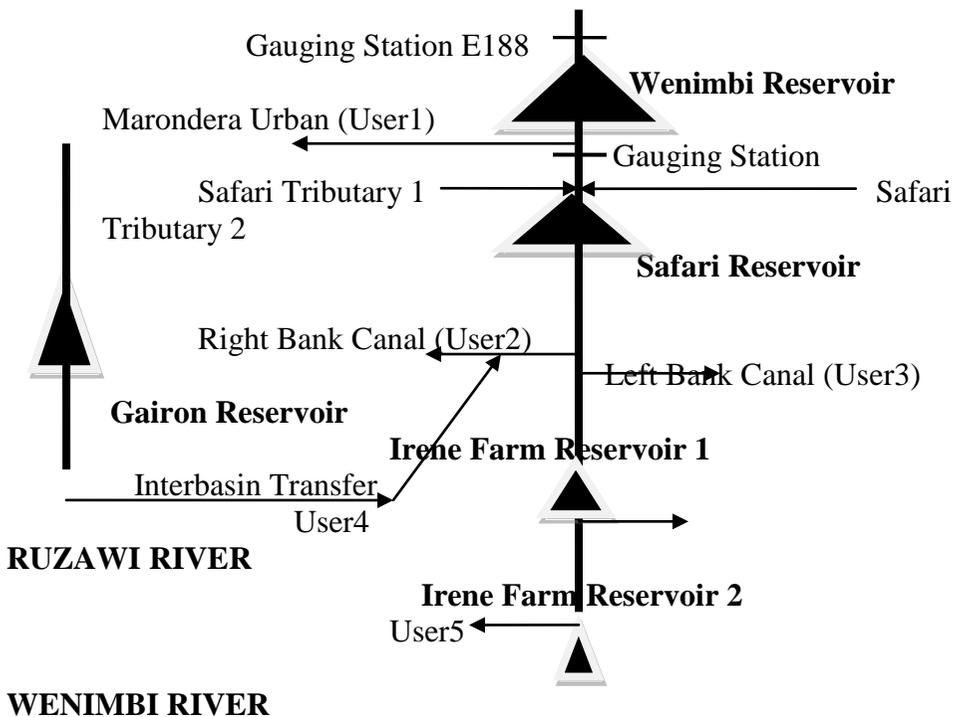
Figure 3: Conceptual Model of the Safari-Igava Water Resources and Uses
