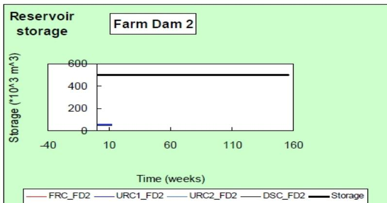
Figure 12. Eirene Farm Reservoir 2 storage at peak demand (Marondera Town water supply connected and 75% irrigation efficiency)
